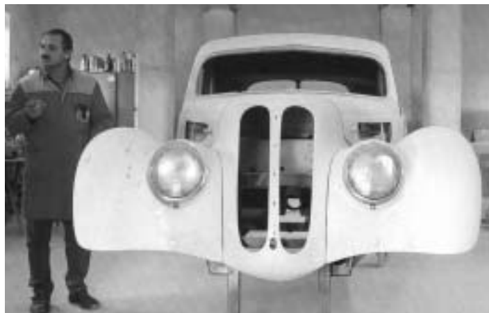
Full body restoration, ready for the paint booth
