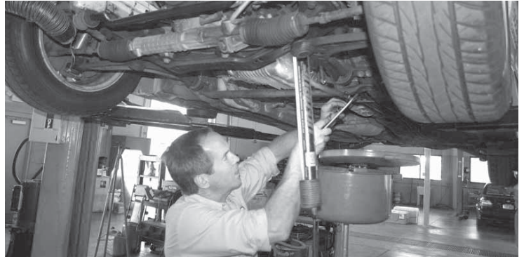
A quick connection down below and it's ready to "Start your Engine" to run the solution through the FI system. Takes about 1 hour start to finish, Mark is really fast.
