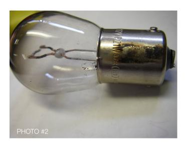
Then I noticed the stain on the bulb base (see Photo #2) and examined the bulb holder, which had partially melted in the area of the bulb-ground contact. The fix was a new bulb holder (63-25-8-375-599, listed as fitting all E39 sedans; list price less than \$10), which was conveniently in stock at my local BMW dealer. Rather than clean up the old bulb and reinstall it, I replaced it with a shiny new one (my guess is that the old bulb was the original on this 1999 Fiver).
