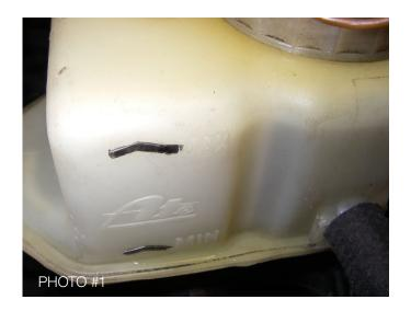
"Max" and "Min" level arrows emphasized with felt-marker ink. You can see that there is considerable room for expansion provided above the "Max" arrow. So, when you are changing your brake fluid, ensure that the level is at, but not above, the "Max" mark, AFTER THE CAP AND LEVEL SWITCH ARE IN PLACE.
